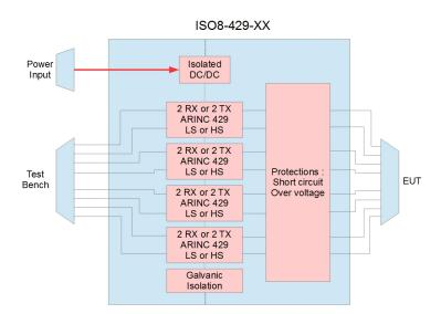
Up to 4 piggy boards with 2Rx or 2Tx channels can be plugged on the carrier board proposing from 8RX/0TX to 0RX/8Tx with all the between configuration. The protection circuits are installed on the carrier, on the Equipment side.
