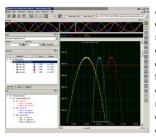
A base license of SBench 6, the easy-to-use graphical operating software for Spectrum cards, is included in the delivery. The base license makes it is possible to test the card, display acquired data and make some basic measurements. It's a valuable tool for checking the card's performance and assisting with the unit's initial
