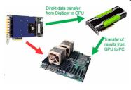
For applications requiring high powered signal and data processing Spectrum offers SCAPP (Spectrum's CUDA Access for Parallel Processing). The SCAPP SDK allows a direct link between Spectrum digitizers and CUDA based GPU cards. Once in the
