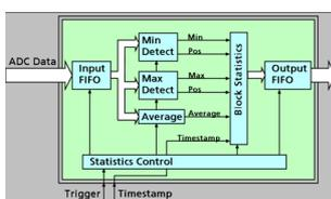
The Block Statistics and Peak Detect Module implements a widely used data analysis and reduction technology in hardware. Each block is scanned for minimum and maximum peak and a summary including minimum, maximum, average, timestamps and position information is stored in memory. The complete averaging process is done inside the FPGA of the digitizer generating no CPU load at all. The amount of data is greatly de-
