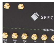
Standard SMA connectors are used for all analog input signals and all trigger and clock signals. No special adapter cables are needed and the connection is secure even when used in a moving environment.
