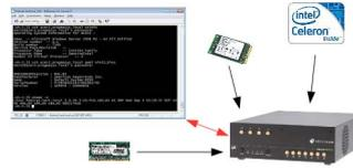
The option turns the digitizerNETBOX/generatorNETBOX in a powerful PC that allows to run own programs on a small and remote data acquisition system. The digitizerNETBOX/generatorNETBOX is enhanced by more memory, a powerful CPU, a freely accessible internal SSD and a remote software development access method.
