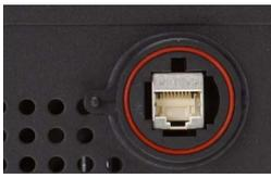
The GBit Ethernet connection can be used with COTS Ethernet cabling as well as special industrial grade Buccaneer Ethernet cables. The integration into a standard LAN allows to connect the digitizerNETBOX/generatorNETBOX either directly to a desktop PC or Laptop or it is possible
