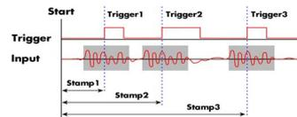
The timestamp function writes the time positions of the trigger events in an extra memory. The timestamps are relative to the start of recording, a defined zero time, externally synchronized to a radio clock, an IRIG-B a GPS receiver.
