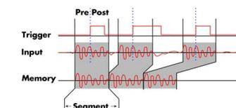
The Multiple Recording mode allows the recording of several trigger events with an extremely short re-arming time. The hardware doesn't need to be restarted in between.
