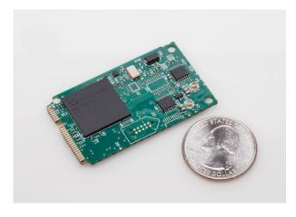
The exact time-of-occurrence of random external events may be captured by using the Event Time input. When the event input is sensed the current time is saved in a buffer for later interrogation by the host. The resolution of the time tag is 100 nanoseconds.
